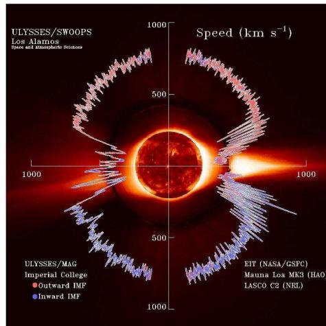
$$B_r(r) = B_{r0} \left(\frac{r_0}{r}\right)^2 \quad B_\varphi(r) = -\frac{\omega r B_r}{v_r}$$
